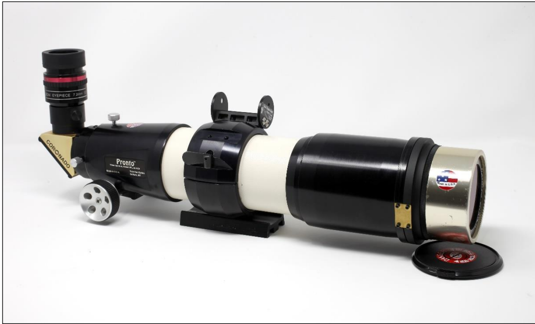
Figure 5- TeleVue Pronto 70mm F/6.8 | SM60 (BF15) – Optimized for H-alpha Solar observation.
