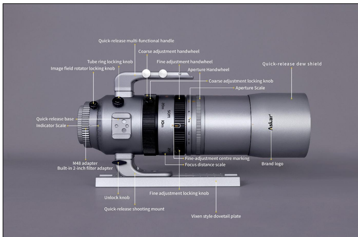
Figure 1 – Askar SQA55 264mm f/4.8 Super Quintuplet Astrograph.
