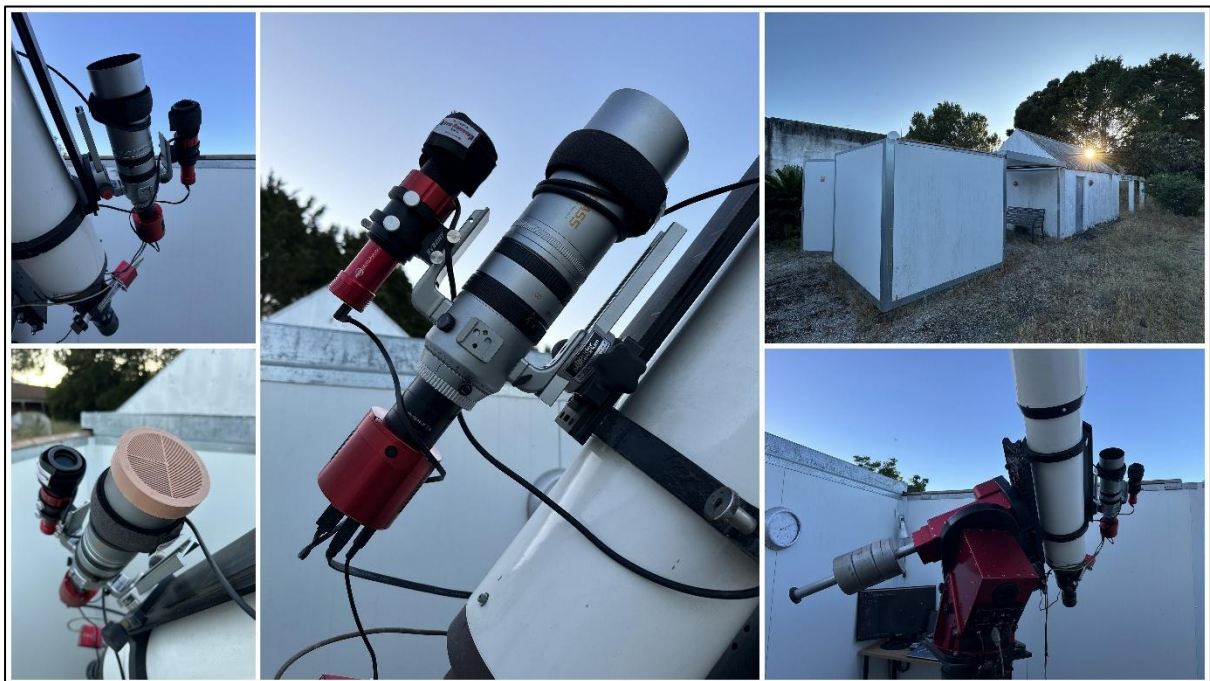
Figure 8 – Askar SQA55 264mm f/4.8 Super Quintuplet Astrograph. Pedro RÉ (2025).
