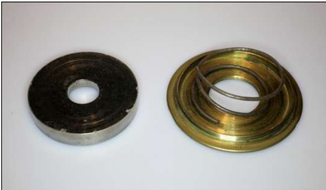
Figure 5- Gregorian Telescope ( circa 1800), speculum mirror. Personal collection Pedro Ré.
