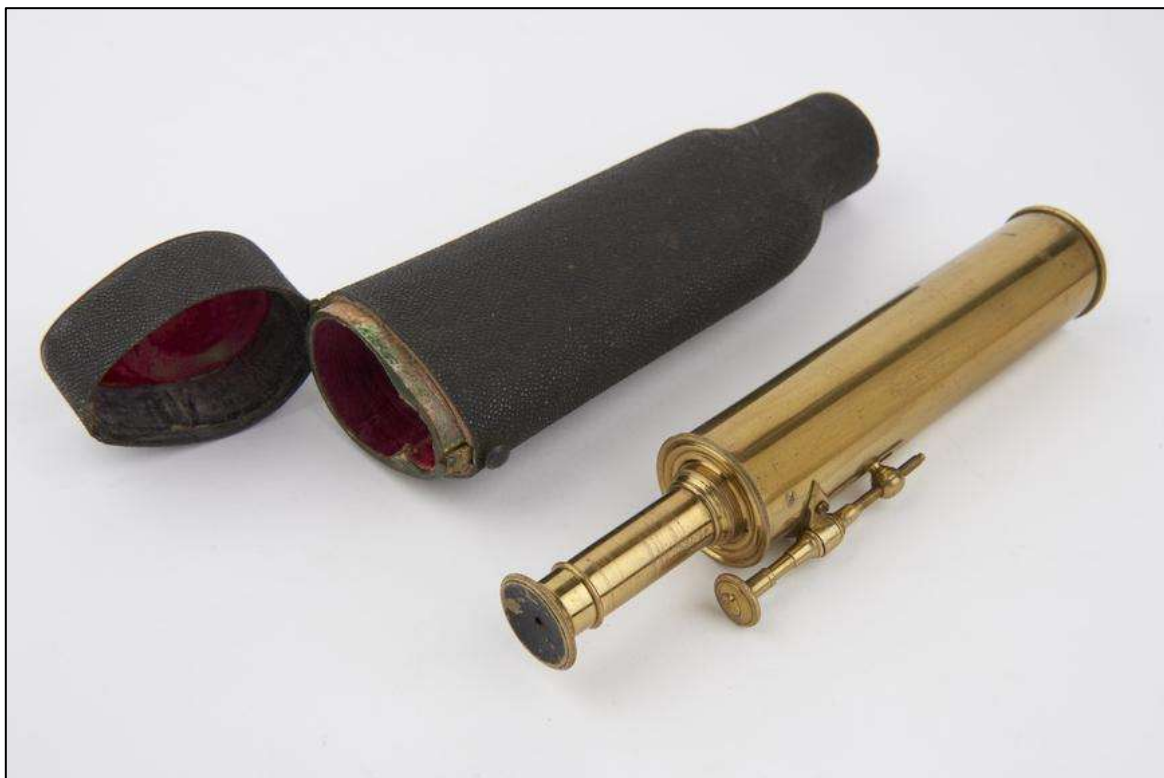
Figure 2 - Pocket brass Gregorian reflecting telescope, speculum mirror, in leather case, unsigned, English, 1740-1800. Science Museum Collection, London.
