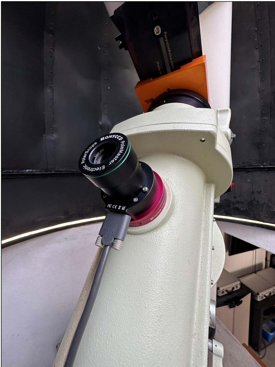
Figure 2- Polemaster installed on a Takahashi EM400 mount.
