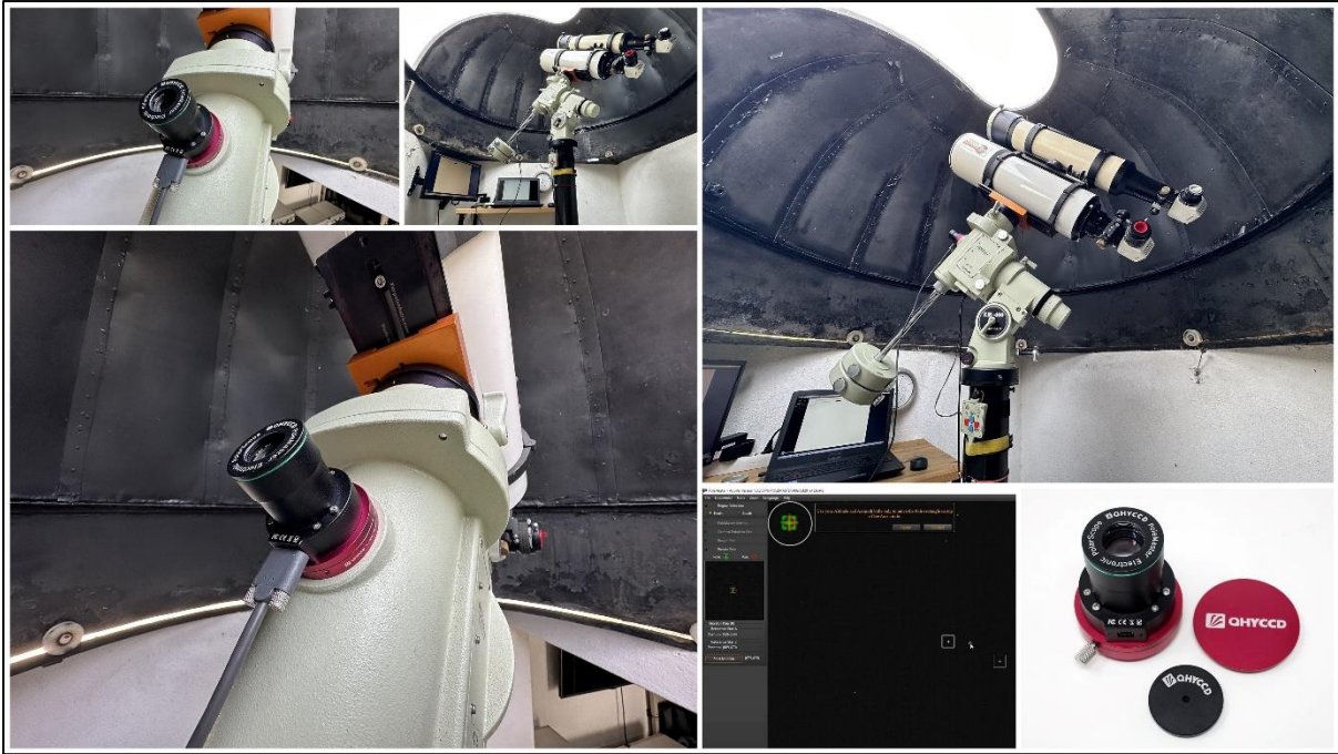
Figure 7- Polemaster, EM-400 mount & dedicated software.
