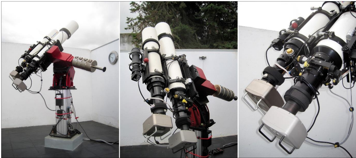
Figure 1- Paramount ME, TMB152 F/7.9, AP130 F/6, SBIG STL11000M (Class 1), SBIG STL1000M (Class 2)
